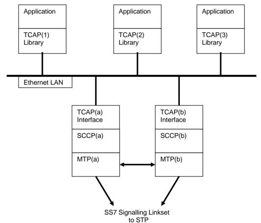
The TCAP interface, SCCP and MTP3 code all reside in the kernel. The application is shown running in a different system, but can run in the same system as SCCP and MTP3 by connecting to 'localhost'.
