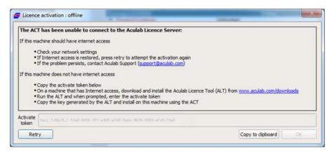
Copy the 'Activate token' and process it with the ALT as you would for an offline 'Install' token. Then install the key returned by the ALT with the ACT. This needs to be performed before the Expiry date or the licence will need to be re-installed.
