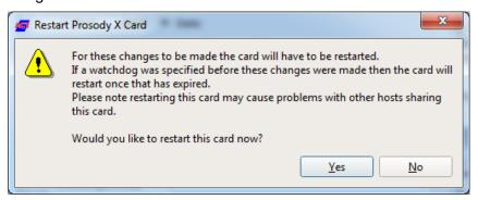
If you are using Edit to configure a Prosody X card for the first time, select 'No'. If you are using the Edit option to change an IP address, the new IP address will not be applied until the Prosody X card has been rebooted, therefore select 'Yes'.
