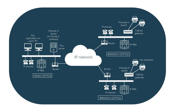
Aculab Cloud, Aculab's Prosody X high density, high performance, intelligent fax boards and Prosody S with T.38 fax software provide the enabling technology for communications system developers to create a variety of fax applications to integrate fax transmission with TDM and/or IP networks.
