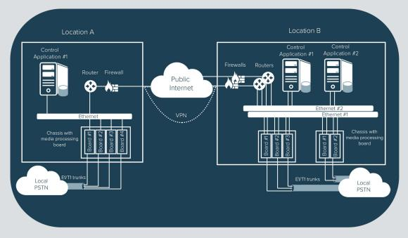
Figure 3 – Architecture of a voice-based solution distributed between remote geographical locations
